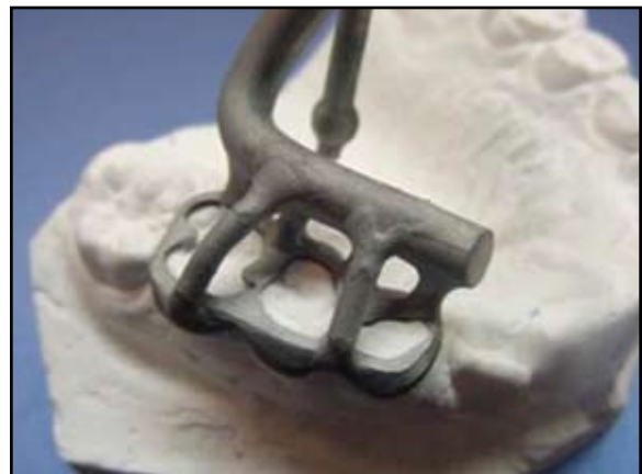
Fig. 2 Metal splint cast from biomedical titanium using lost-wax-fusion technique.
